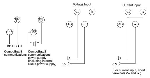
For current input, short terminals V+ and I+. Use the short circuiting fitting provided to accomplish this.
