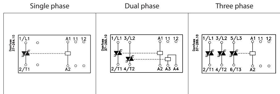
Terminals 11 and 12 have no connection to the internal circuit but are intended for connection to an optional overload protection (see overheating protection instruction, page 4).
