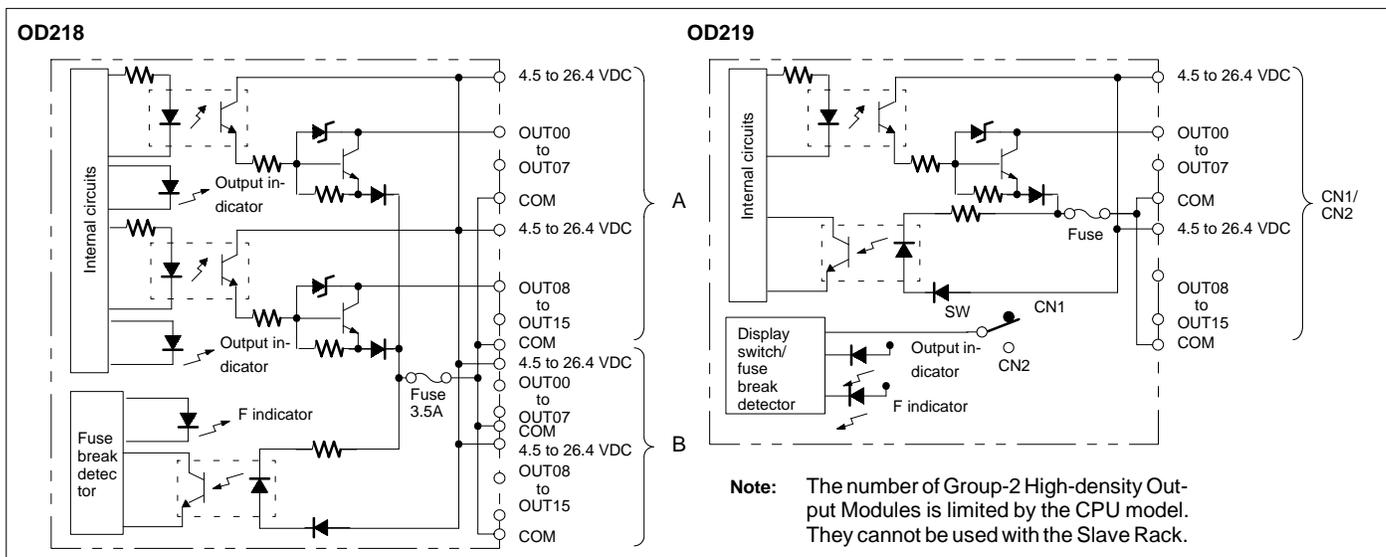
**Note:** The number of Group-2 High-density Output Modules is limited by the CPU model. They cannot be used with the Slave Rack.
