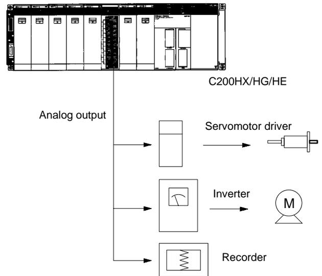
Converts 12-bit binary data into analog signals (voltage or current) for output to external devices.
