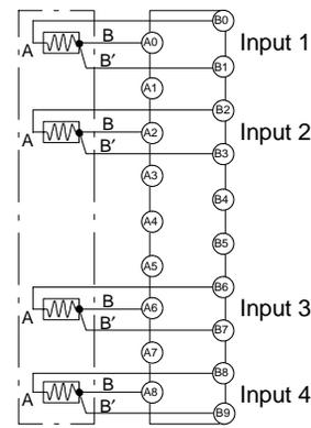
**Note:** A cold junction compensating circuit, whose precision is adjusted together with the Module, is provided between the B4 and B5 terminals of the C200H-TS001 (for thermocouple).
