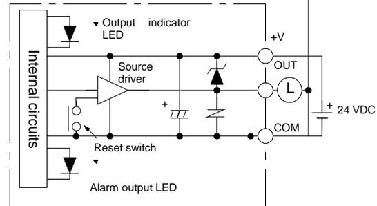
Transistor Output (Protective Circuit for Load Short-circuit): OD216/OD217
