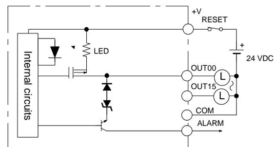
**Note:** Fuse blowout detection circuit: The F indicator is lit and the 08 bit turns ON. The 08 to 15 bits cannot be used as ordinary IR bits.
