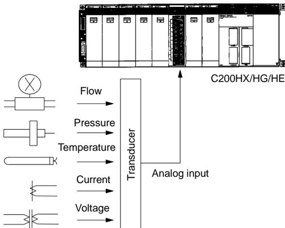
Analog signals, such as voltages and currents, are received from various sensors through the maximum of 8 inputs (AD002) and converted into 12-bit binary data.
