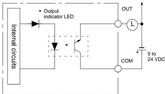
Transistor Output (Source Type with Protective Circuit for Load Short-circuit): OD21A
