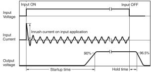
Note: Twice the normal inrush current will flow during parallel operation or for backup operation. Also, if crossover wiring is used for N number of Power Supplies, an inrush current of N times the inrush current for a standalone Power Supply will flow. Therefore, check the fusing characteristics of fuses and operating characteristics of breakers making sure that the external fuses will not burn out and the circuit breakers will not be activated by the inrush current.
