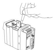
Press the button to eject the holder. Mount the SIM card in the holder and make sure it is correctly installed before it is pushed back into the modem.
