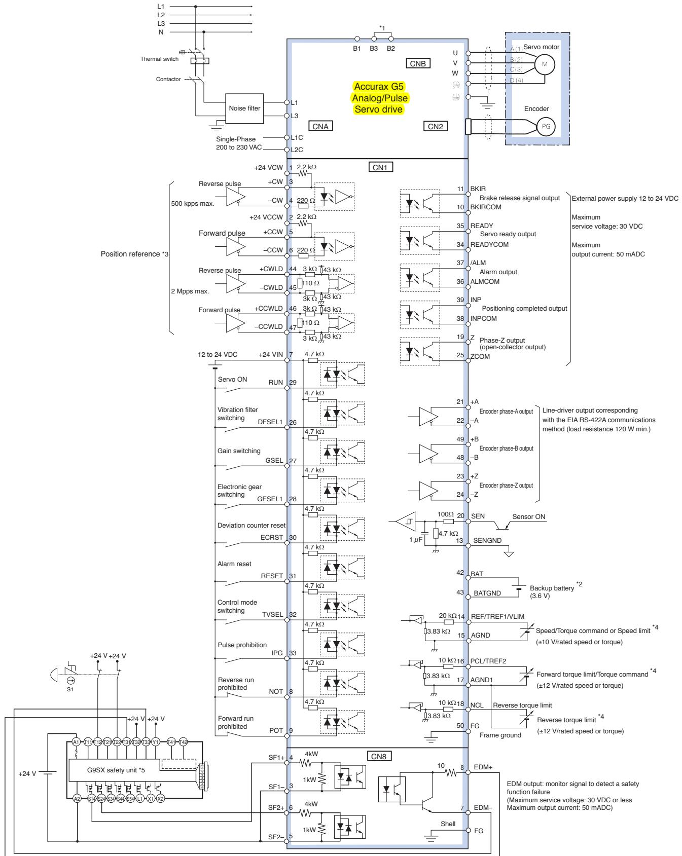
\*1 For servo drives from 750 W, B2 and B3 are short-circuited. If the internal regenerative resistor is insufficient, remove the wire between B2 and B3 and connect an external regenerative resistor between B1 and B2.
