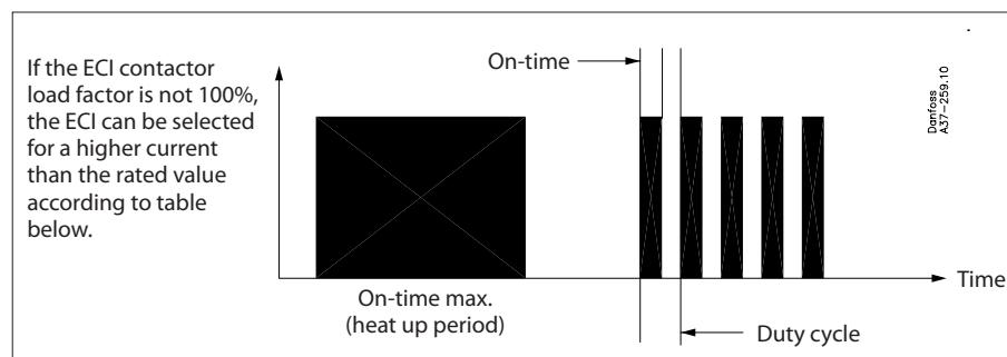
$$\text{Load factor} = \text{On-time} / \text{duty cycle}$$
