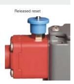
If the rope stretching indicator is in the correct operation area, it is possible to close the electric safety contacts pulling the blue reset button. The green ring signal allows to know the switch condition quickly.
