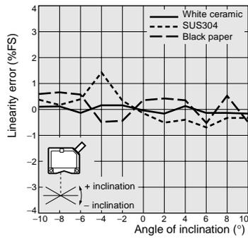
Linearity Characteristic for Different Materials (Reflective Sensors)
