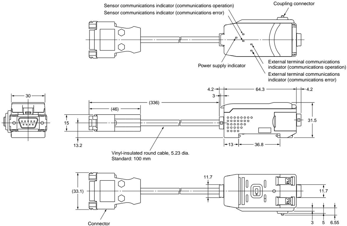
**Cables with Connectors on Both Ends (for Extension)**
