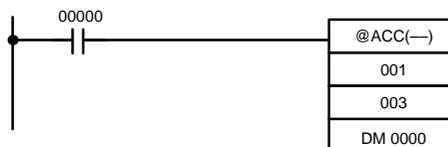
When IR 00000 turns ON, ACC(—) begins decelerating the port 1 pulse output at about 1,000 Hz/4 ms until it reaches the target frequency of 5,000 Hz.
