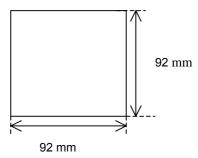
Install the NT2S from the front of the panel. (Make sure that the gasket is properly mounted)
