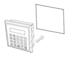
Secure the NT2S, with the provided attachments to the panel.
