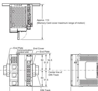
Note: For dimensions with the communications cable connected, refer to NX-series User's Manual Safety Control Unit/Communication Control Unit (Cat. No.Z395)
