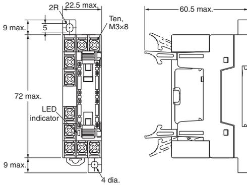
**Note 1:** The front view shows with the finger cover removed.
