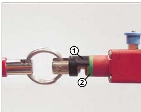
Stretch the rope connected to the switch, until the end of the indicator (1) reaches about the middle of the green ring (2).
