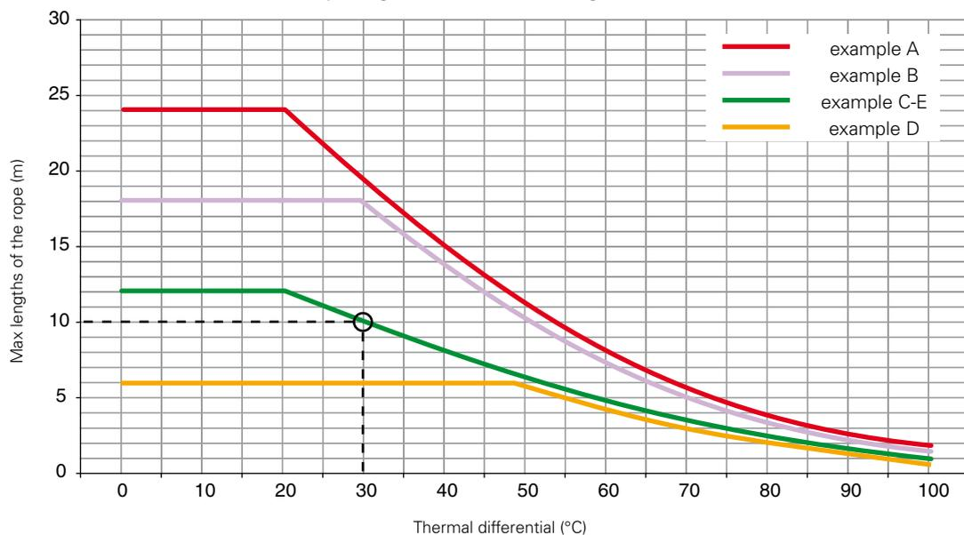
In the diagram, the suggested max. rope lengths with regard to changes of temperature (thermal differential) to which the switch is expected to be exposed in the working area are indicated.
