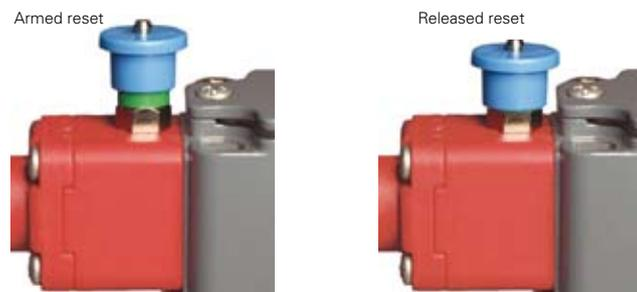
If the rope stretching indicator is in the correct operation area, it is possible to close the electric safety contacts pulling the blue reset button. The green ring signal allows to know the switch condition quickly.
