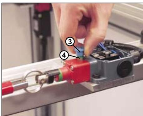
Pull the knob (3) in order to close the safety contacts inside the switch. Below the knob a green ring (4) will be disclosed.
