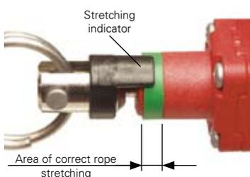
All switches are provided with a green ring that shows the area of the correct stretching of the rope. The installer has only to stretch the rope until the black indicator will be in the middle of the green area. In this position it is possible to reset the switch, pulling the reset button, and to close the electrical safety contacts.
