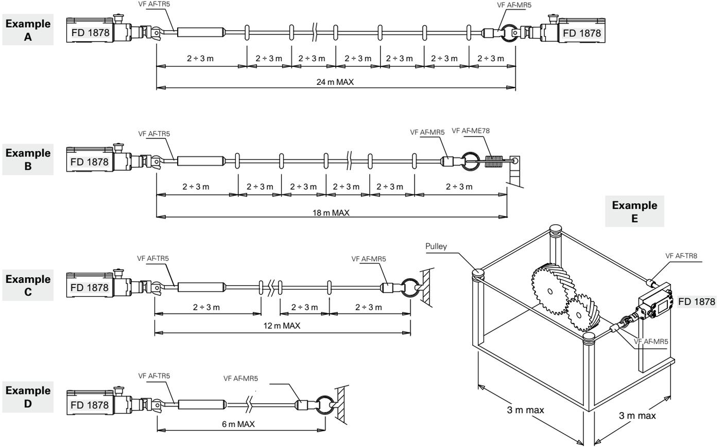
Application examples and max rope length for switches with transversal heads
